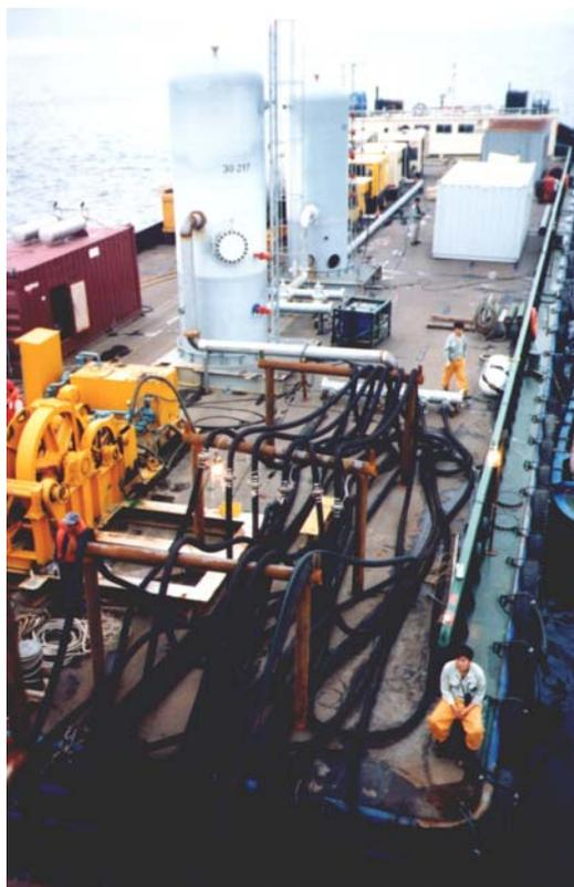
The mooring system required to moor the Spacer and control the Molikpaq during mating was pre-installed on the alternative mooring site. Bad weather frequently hampered the anchor lay operation. Once all anchors were installed, some failed the 100% pre-load test, requiring the piggy backs of large concrete blocks.
