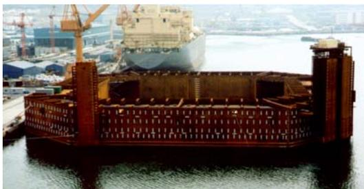
The Spacer hull was subdivided into 8 main ballast tanks and 8 corner tanks. A hydraulic operated valve system was installed for gravity ballasting. Deballasting was effected by compressed air, provided by a bank of rental compressors, mounted onto a barge. The compressed air was forced through the vent pipes via a manifold. The Ballast Control Container was mounted on the center buoyancy tower, where the valves for the vent pipes and air manifold were also located.
