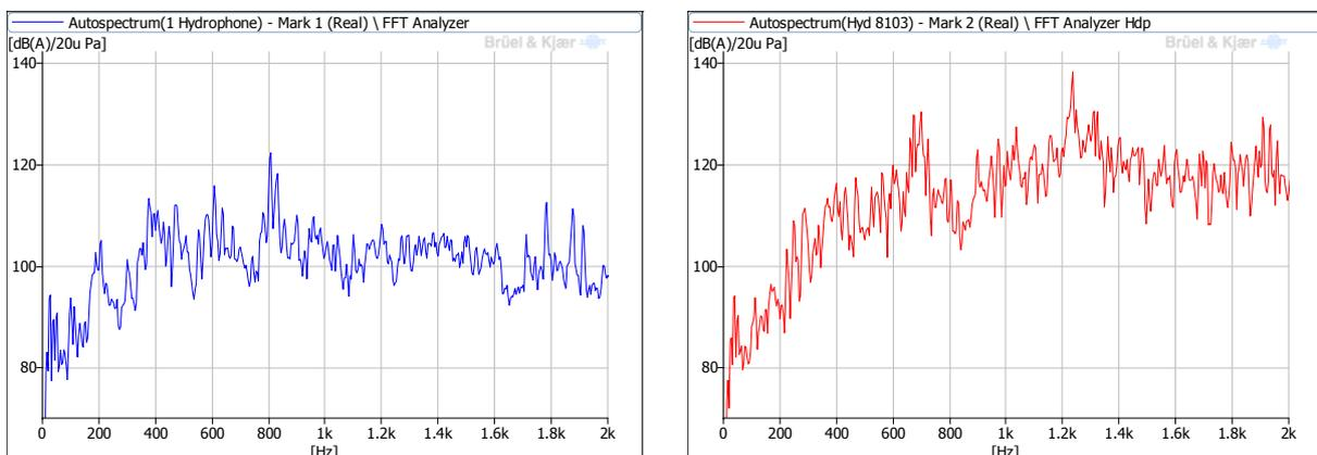
Figure 8. W6L34DF cam-gear cover inside A-weighted sound pressure level comparison, diesel 100% load, 750 rpm. Left, standard gear train; Right, anti-backlash gear train.
