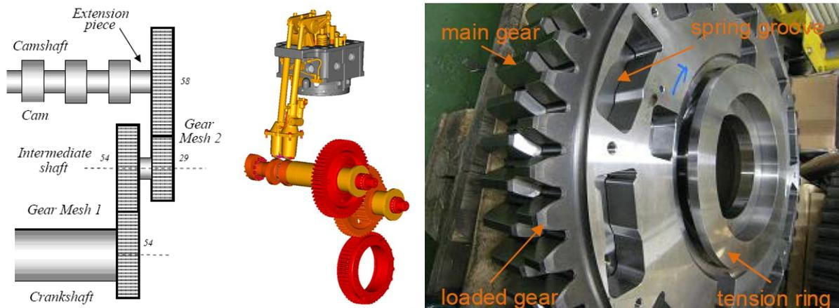
Figure 1. Left, schematic picture of the gear train system; Middle, W32 gear train model; Right, two parts of the anti-backlash large intermediate shaft gear.
