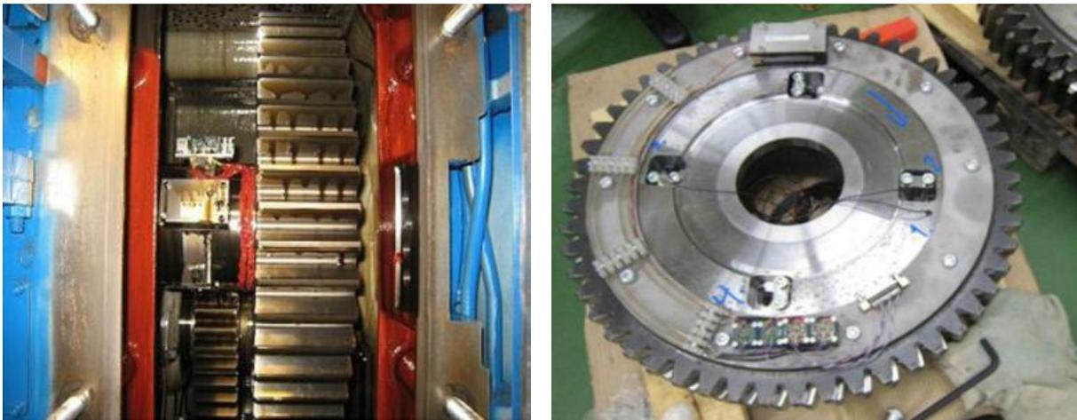
Figure 2. Left, strain gauge on the extension piece of the camshaft next to the cam gear; Right, acceleration sensors setup for the anti-backlash large intermediate shaft gear.
