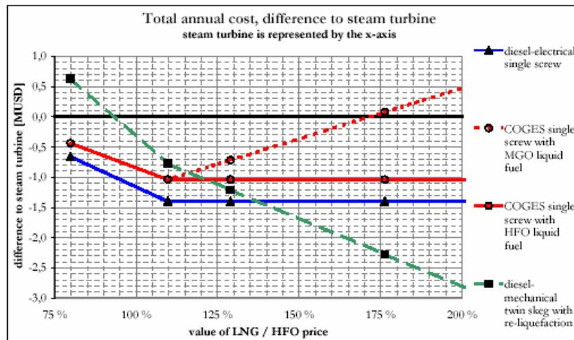
**Figure 9 Total annual cost, versus the ratio of LNG value and HFO price, presented as difference to the steam-mechanical machinery**
