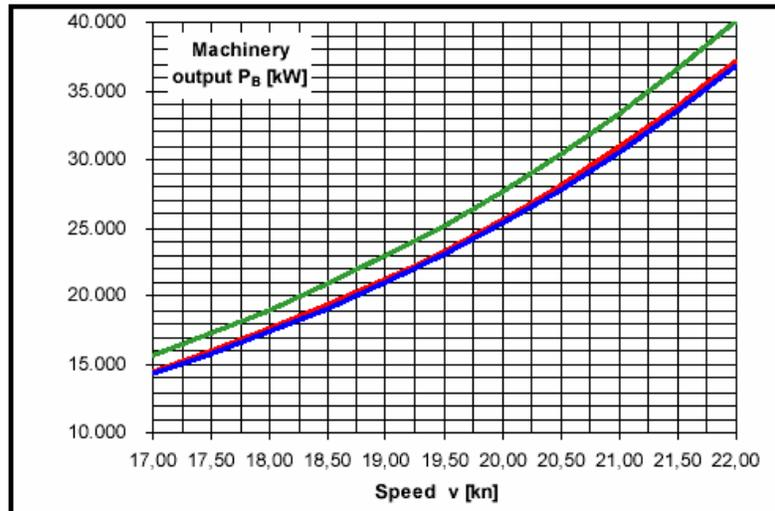
Figure 3: Predicted Brake Power Requirements
