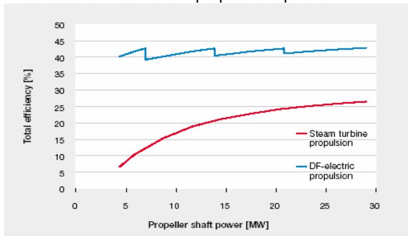
Fig. 2 Efficiency comparison between DF-electric and steam turbine propulsion for the case quoted in this article.
