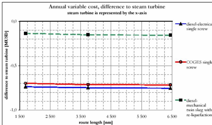
**Figure 6 Recurring annual variable cost, versus route length, presented as difference to the steam-mechanical machinery**
