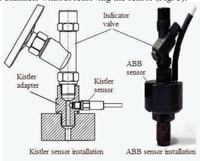
Fig. 3. Pressure sensors monted before indicator valves
