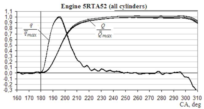
Fig. 7. Heat release characteristics referenced to maximum values  $q_{max}, Q_{max}$ , designated from indicator graphs measured on the indicator valves of low speed diesel engine (sea trials) Sulzer 5RTA 52
