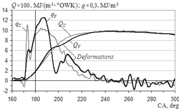
Fig. 6. Heat release characteristics based on the indicator graph of medium speed engine 6AL20/24: measured in the cylinder –  $q_c, Q_c$ , measured on the indicator valve –  $q_v, Q_v$ :  $q$  – intensity of heat release,  $Q$  – heat release
