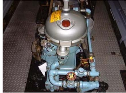
The objective of the task is to remove the build up of sludge, dirt, grim that gathers on the individual disc during the separation procedure. This debris must be physically taken off.
