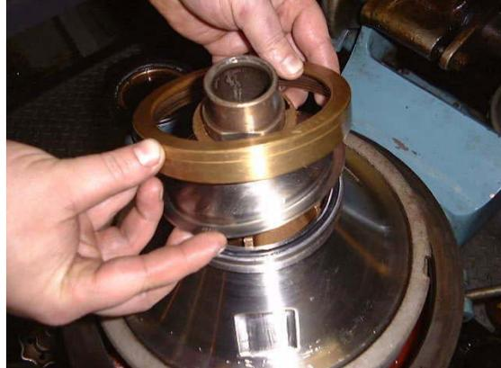
15) Release locking screws and rotate bowl assembly to check for trouble (grinding, roughness etc) it should be smooth. Close the unit's lid and secure both clamps hand tight.
