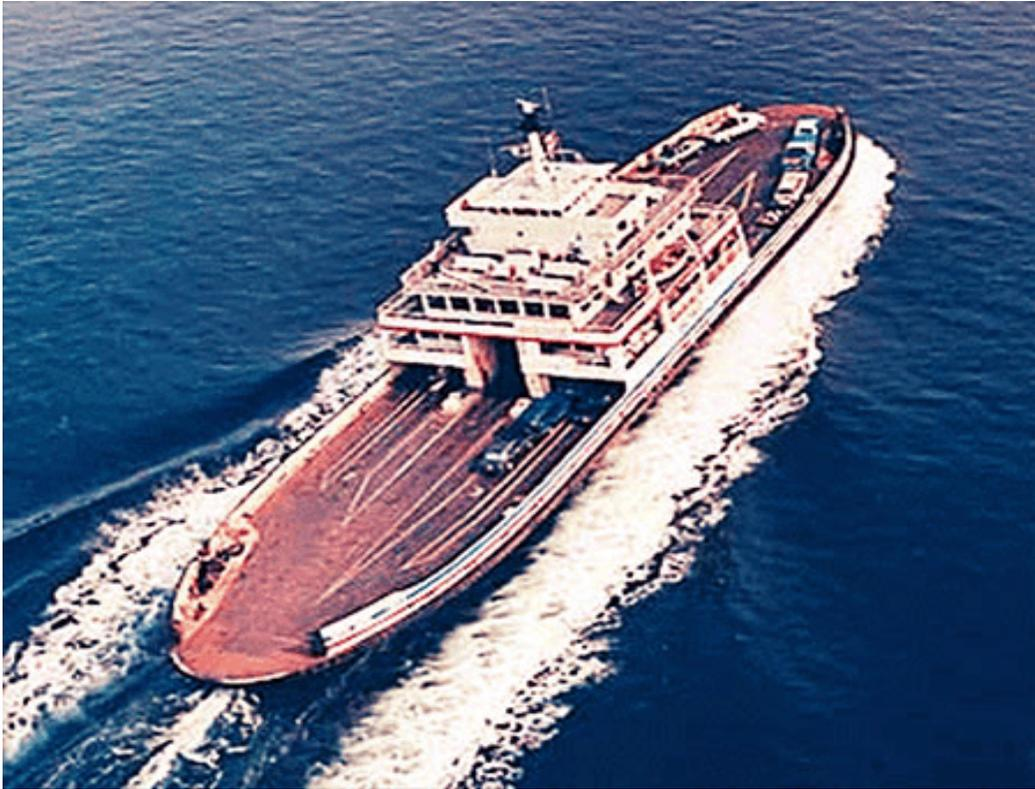
**Figure 1.** Aerial view of vessel showing wheelhouse, vehicle deck and double ended features.
