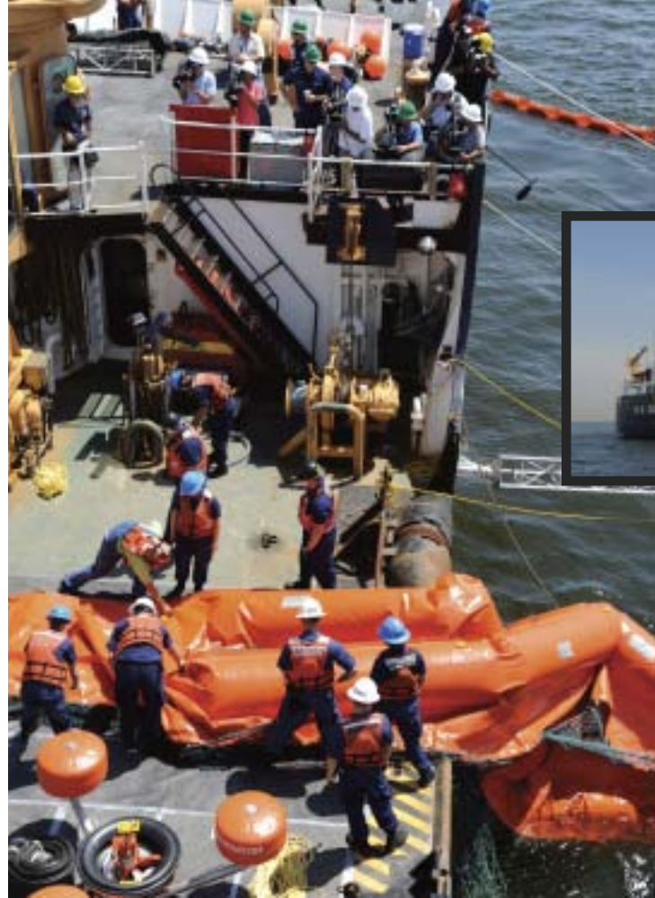
CGC Juniper's spilled oil recovery system.
