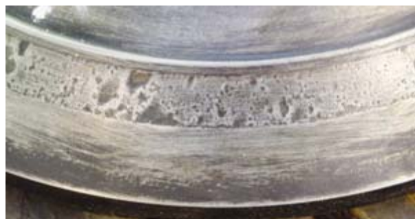
Figure 03: Typical dent marks of the seat of a valve spindle (MC60-type Nimonic after 8,300 hrs)
