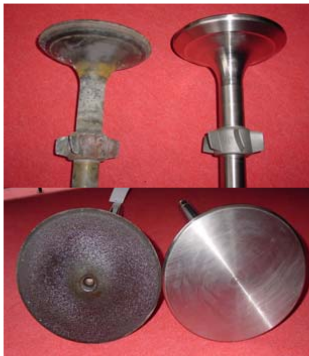
Figure 15 a/b: Nimalike spindle before and after remanufacturing
