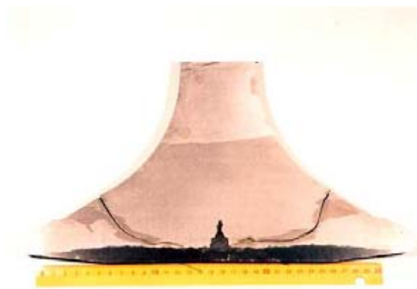
Figure 13: Macro cut through the center of a valve head (RTA62 Nimonic-type 6,430 hrs after repair)
