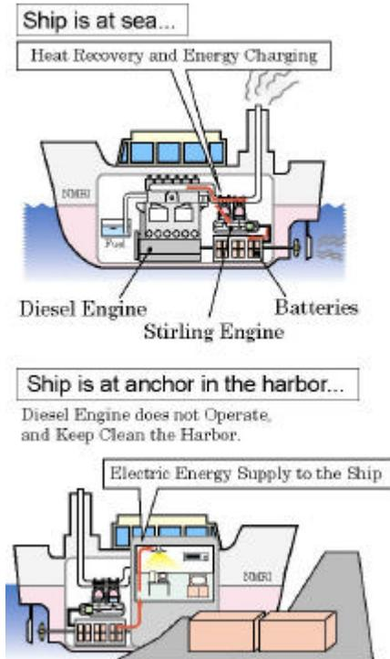
Fig. 6, Waste Heat Recovery System to Keep Clean the Harbor Area
