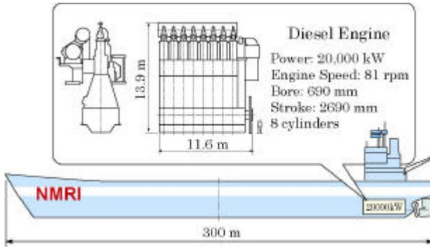
Fig. 1, Marine Diesel Engine for Large Freight Ship
