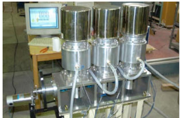
Fig. 8, Photograph of the Prototype Stirling Engine
