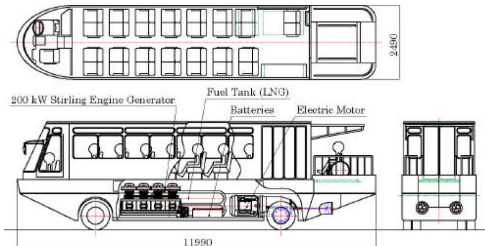
Fig. 4, Conceptual Drawing of Sightseeing Amphibious Vehicle
