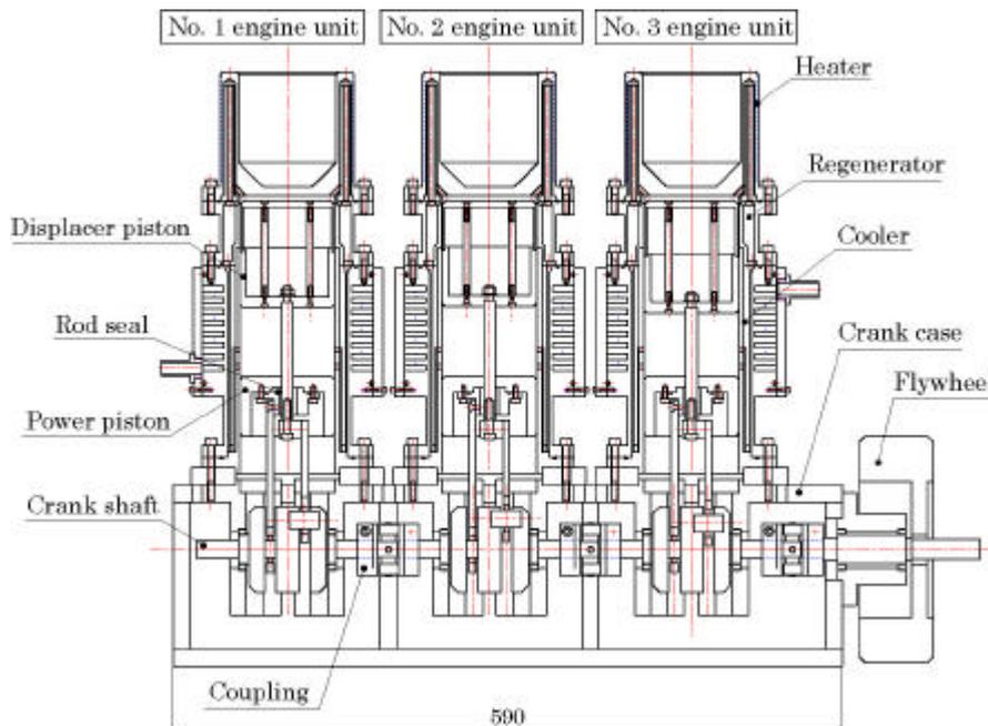
Fig. 9, Schematic View of the Prototype Stirling Engine
