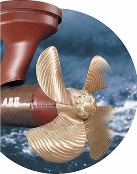
System construction is straightforward, consisting of a Propulsor Module and a Steering Module, providing unlimited azimuthing angles. The Propulsor Module incorporates an ultra-efficient permanent magnet synchronous motor with a fixed-pitch propeller mounted directly to the motor shaft. The compact motor is directly cooled by surrounding seawater, allowing for a simple mechanical construction and a slim pod with superb hydrodynamics.
