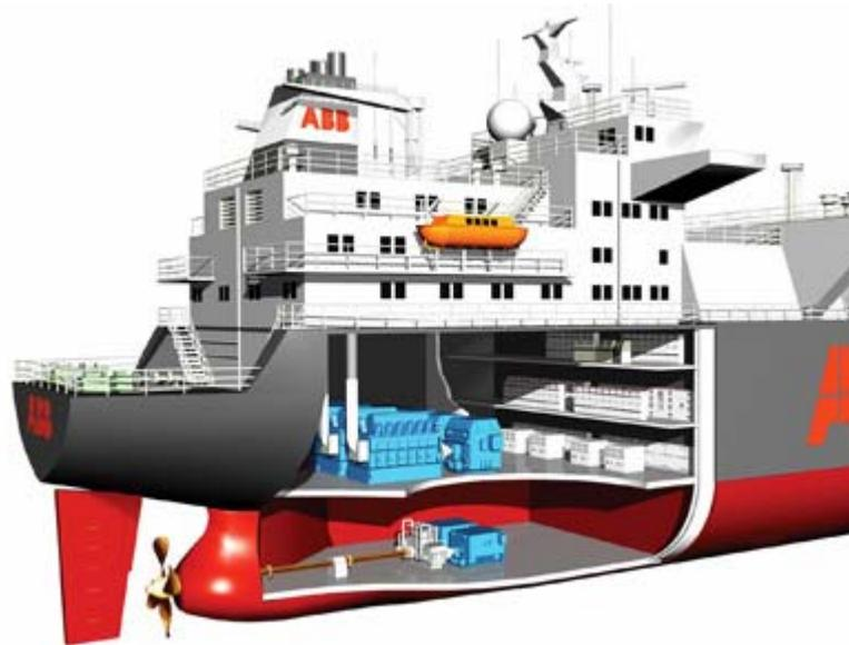
Electric propulsion system for LNG carriers
