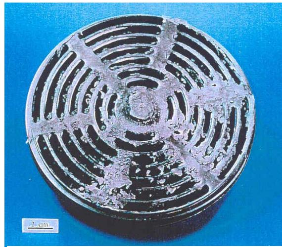
Fig 2 - Plate valve from a PP process compressor - For contaminated gases poppet valves are more suitable
