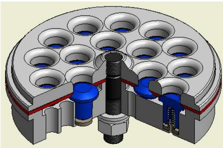
The COP<sup>®</sup> Valve is a poppet type valve that does not require any rework of the seat. The actual valve seat is the seat plate that is replaced when worn. Therefore, the overhaul of a COP<sup>®</sup> valve is very simple: Cleaning and replacing parts is all that is needed. The wear parts, poppets, springs, lift washers and seat plates are easy to stock and not expensive. The seat plate does not have to be replaced at each overhaul.
