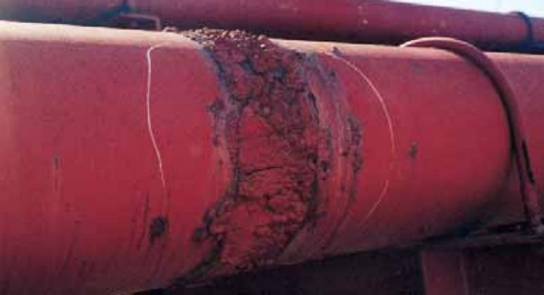
Image: Pipe corrosion
