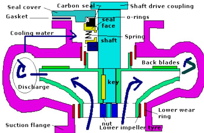
Shown above is a cross section through a vertically mounted centrifugal pump.
