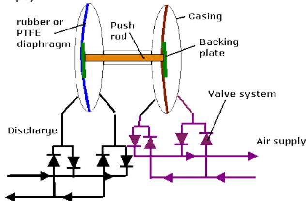
This air supply valve assembly normally takes the form of a shuttle valve.
