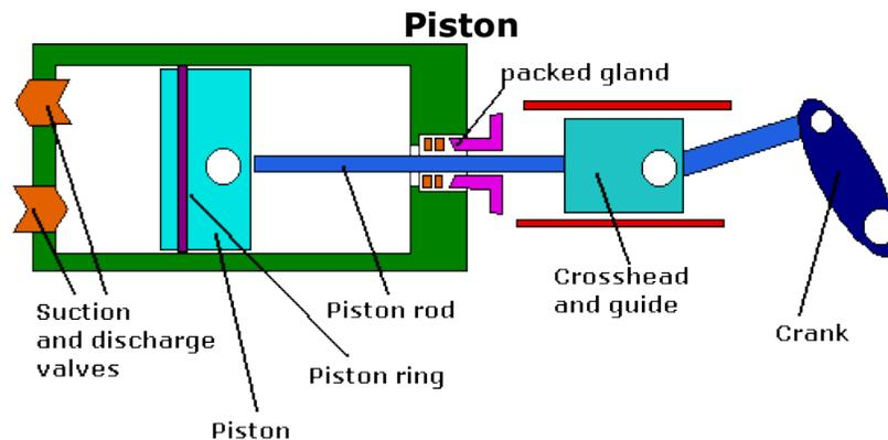
This type of pump is in common use as a bilge pump or tank stripping pump. For older vessels steam driven varieties served in almost all systems.
