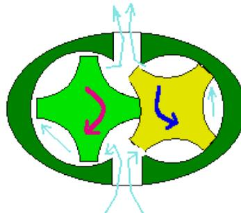
The pump shown above is of very common design. It is used for pumping many types of liquid and gas and is capable of delivering at very high pressures. This makes it suitable for hydraulic supply.
