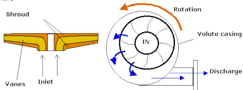
The kinetic energy of the fluid flowing through the impeller is converted to pressure energy by the shape of the volute casing. For high pressure pumps such as boiler feed pumps a diffuser ring is fitted in the casing which converts a greater portion of the pressure energy allowing greater pressures to be generated.
