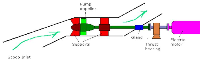
These tend to fit somewhere between positive displacement and centrifugal. They tend to be of the very large capacity type and are often seen in use for supply of cooling water for steam ship condensers. This is particularly true where 'scoops' are employed as the axial flow pump offers very little resistance to flow when idling.
