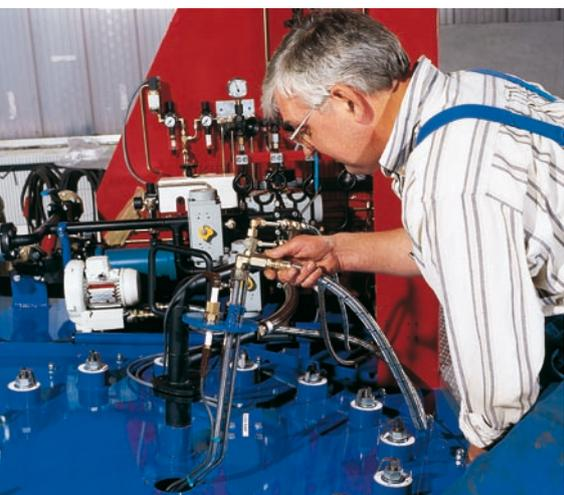
*KBSD™ steam atomizing burner for MISSION™ OL boilers.*
